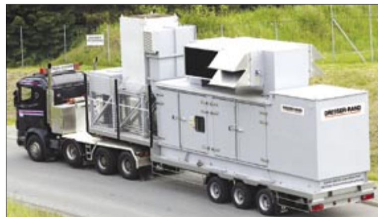
Dresser-Rand's mobile power generating unit
