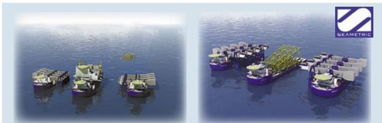
Topside removal of SeaMetric's Twin Marine Lifter
